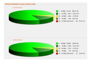
Highest speed, 72 mph outgoing, midnight Saturday. Cars pinged = 3 in half hour section. There is less than 1% at 40-45mph and also 45+mph. The 30-35 mph is the highest offending bracket with 15% of total cars.
